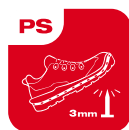
PS Non-metallic perforation- resistant inserts and insoles
